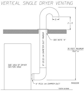
NOTE A: OPENING MUST BE 2-INCHES (5.08 cm) LARGER THAN THE DUCT (ALL THE WAY AROUND). THE DUCT MUST BE CENTERED WITHIN THIS OPENING.
